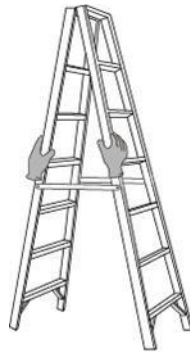
Figure 1- 5 Ensure ladder is held firm
